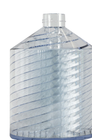
CellScrew CS6K Working Volume: 250-800 mL Growth Area: 6,066 cm 2
