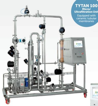
The TYTAN series is based on Microfiltration and Ultrafiltration techniques and operates in the low pressure range of 1-5 bar.
