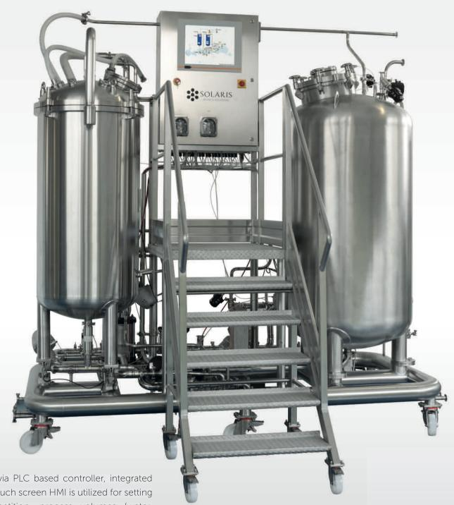
Processes are managed via PLC based controller, integrated to the CIP/SIP unit. The touch screen HMI is utilized for setting up: task sequencing/repetition, process volumes (water, WFI, etc.), detergent dosages, CIP fluid temperature, wash pressure, purging (drainage of equipment and CIP/SIP unit with compressed air), etc.
